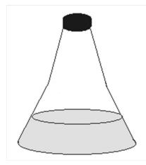
Air pressure 101.3 kPa + 3 kPa from the evaporation of water = about 104 kPa total pressure
