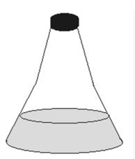
Air pressure 101.3 kPa + 10 kPa from the evaporation of propanone = about 111 kPa total pressure
