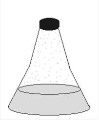
Air pressure 101.3 kPa + 30 kPa from the evaporation of propanone = about 131 kPa total pressure
