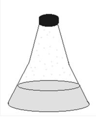
Air pressure 101.3 kPa + 8 kPa from the evaporation of water = about 109 kPa total pressure
