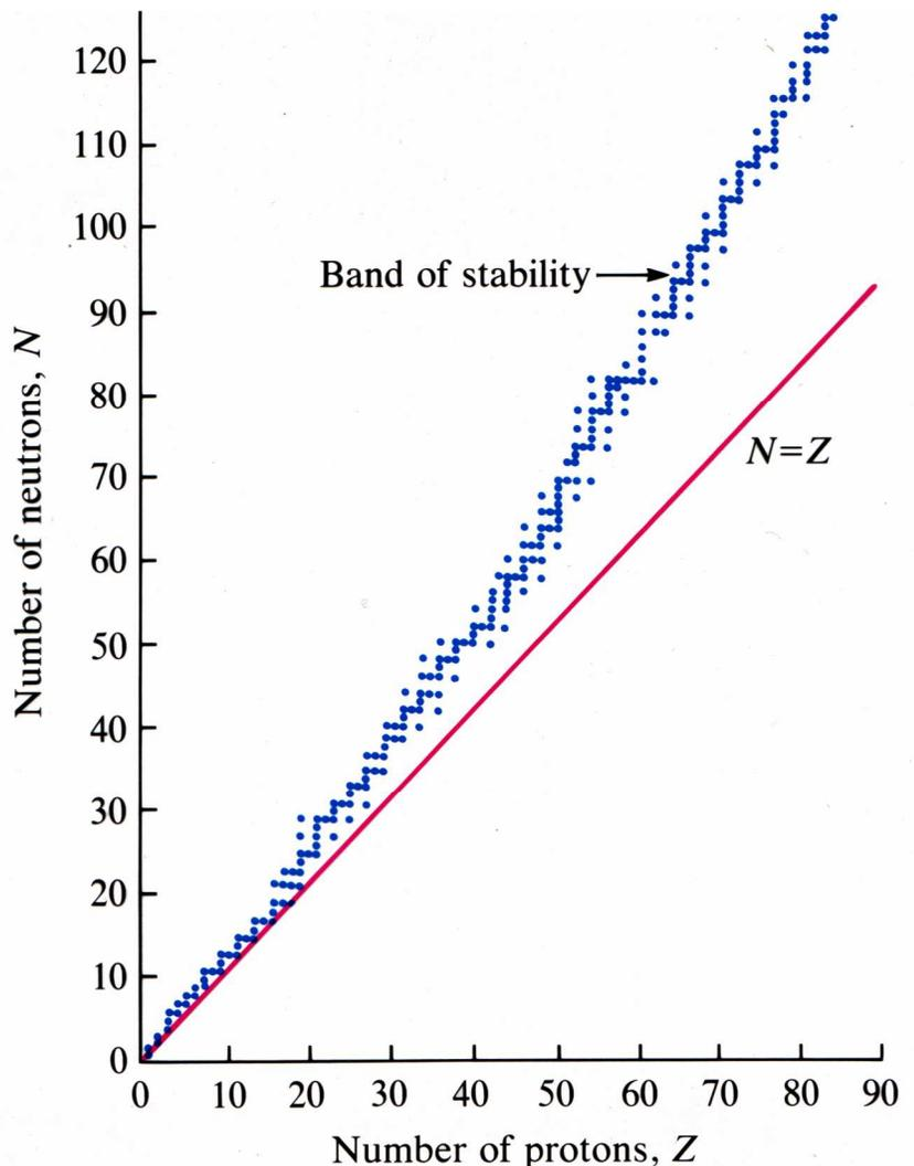
To become stable, these unstable nuclei will emit radiation, parts of their nucleus, to change this ratio of neutrons to protons to some other, hopefully more stable ratio. Sometimes an unstable atom only emits radiation particles one time, and they get a stable nucleus and the radioactive part of their "life" is over. Sometimes it takes more than one step, it must emit radiation more than one time, to keep changing until it gets stable.
